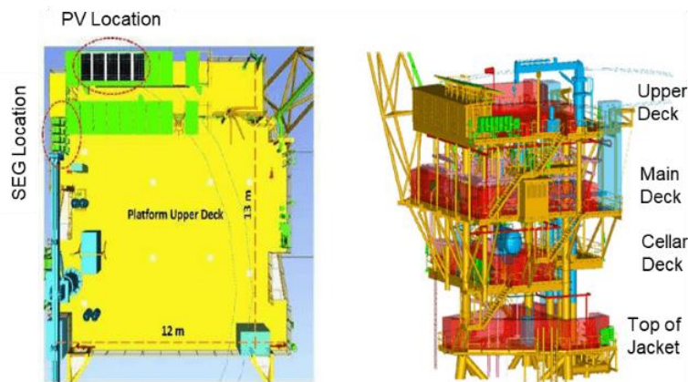
Figure 5. Placement of SEG and PV at the Upper Deck
