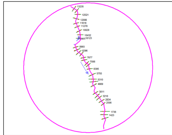
Figure 3. Geometric data of Study River showing river line and cross-sections (RS)
